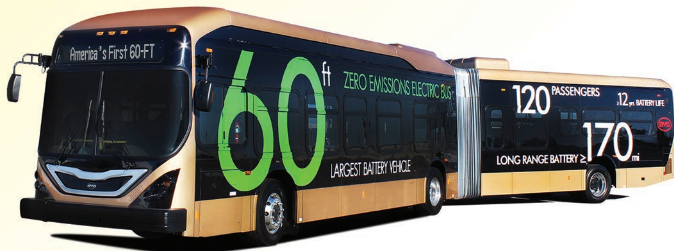
BYD 60-foot, pure electric articulated bus, with a 270 kilometer driving range and that requires only three hours to fully charge
