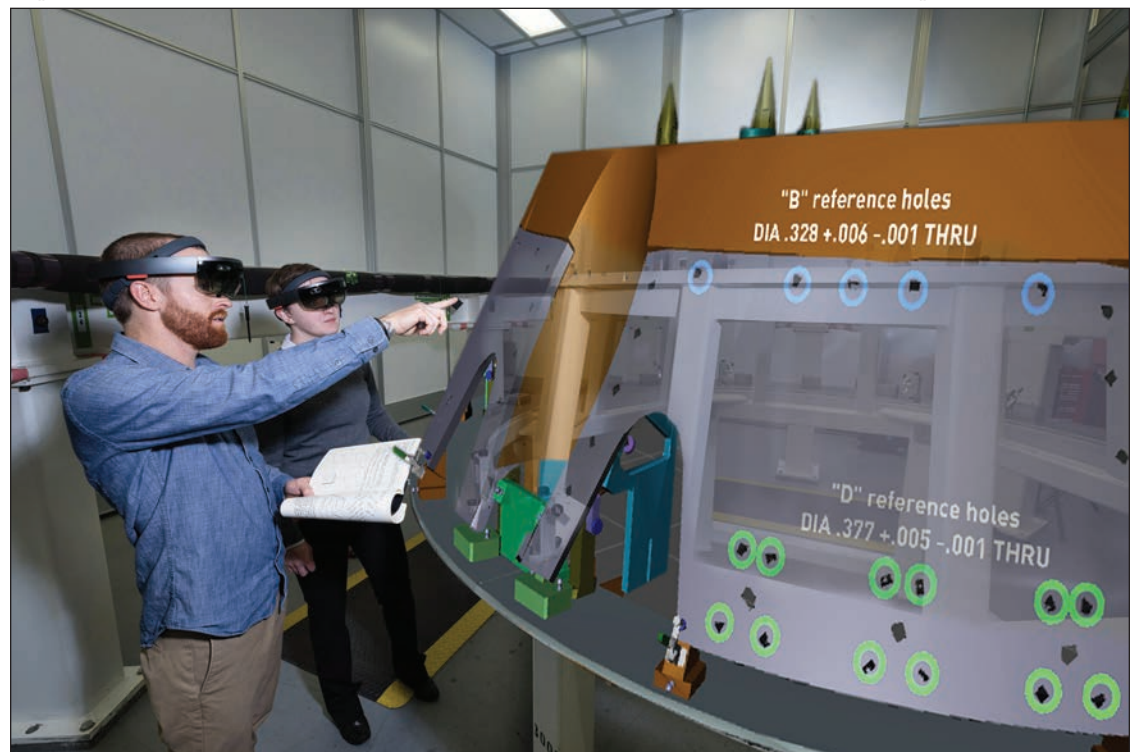
Lockheed Martin technicians use augmented reality to train on an assembly for NASA's Orion spacecraft. AR can reduce the timeframe for complex assemblies by as much as 80-90 percent.
