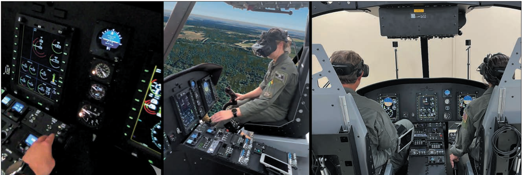
Multi-place Mixed Reality (MPMR) – Integration of real-world avionics within a virtual environment
