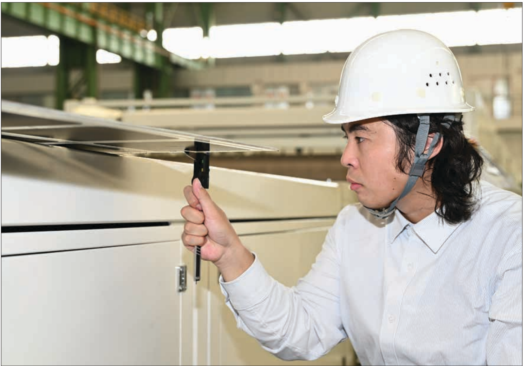
During the development of the tablet pressing technology, every step is meticulously controlled. The image shows the measurement of the edge thickness of a finished photovoltaic panel. Precision is the guiding principle, and perfection is the goal.
